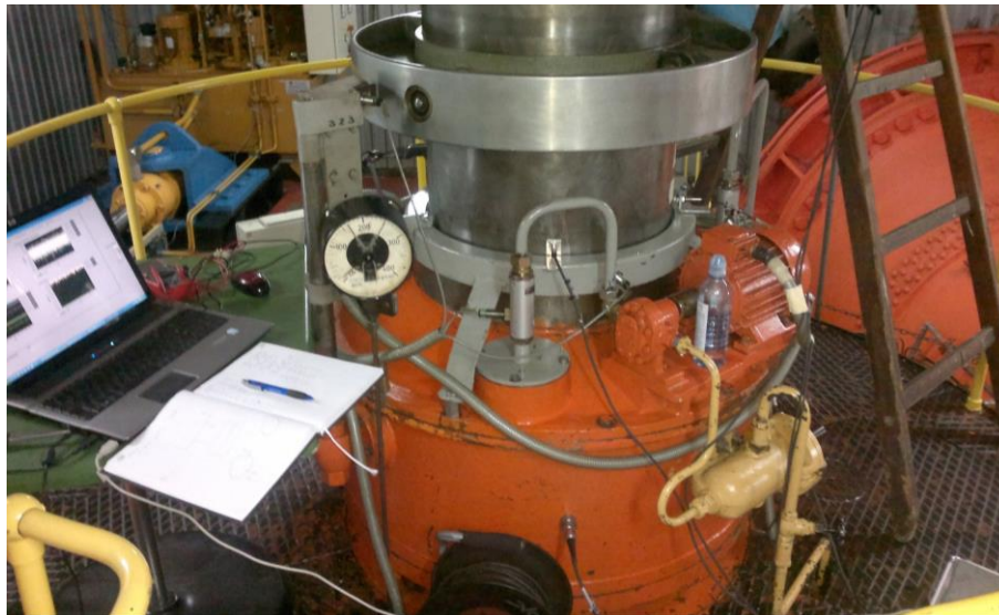
Fig. 3 Sensors at TGB along with the laptop used for measurements.
